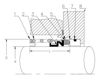
Figure 13: Spring holder configuration
