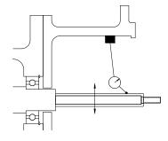
Figure 3: Bearing Fit
