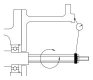
Figure 4: Bearing Frame Perpendicularity
