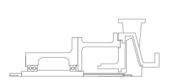
Figure 8: Fully assembled pump without seal
