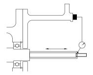
Figure 5: Axial Shaft Movement
