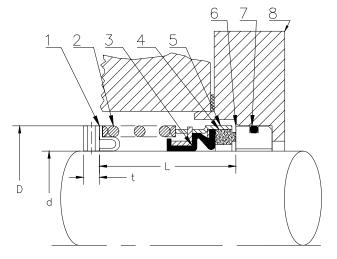
Figure 14: Set screw collar configuration
