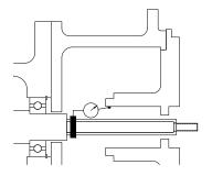
Figure 6: Seal Chamber Bore Concentricity
