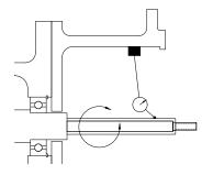
Figure 2: Shaft Runout
